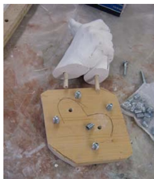
#4. The metal inserts attached to the base.
