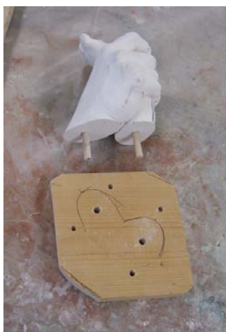
#2. The base with holes to fasten the model and the inserts.
