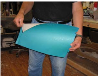
#12. A printer's plate that makes excellent shims.
