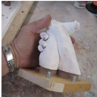
#6. The clay "donuts" in place between the base and the model.
