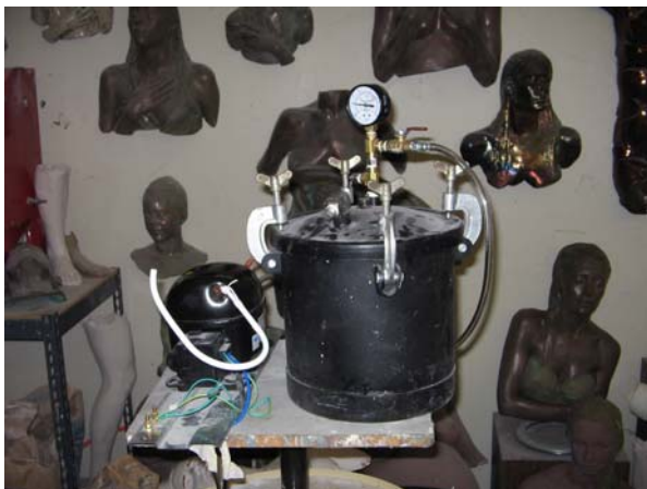
The RU attached to a pressure chamber
