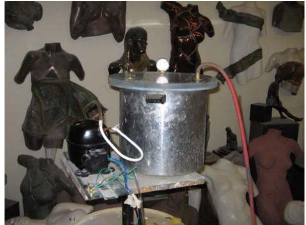
The RU attached to a vacuum chamber
