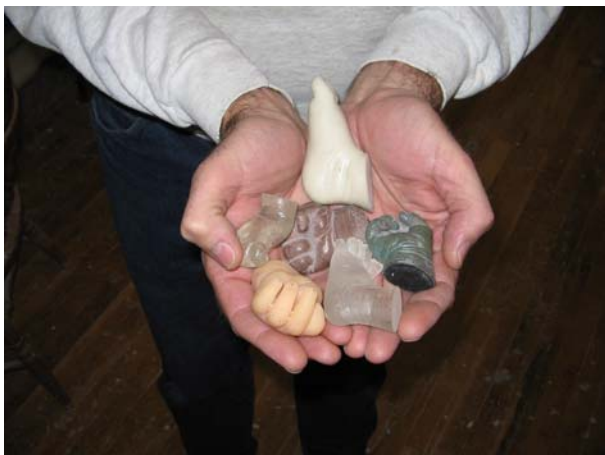
Infants' hands and feet in clear polyester resin, clear polyurethane resin, metallic Forton MG, metallic polyurethane resin, and clear polyester resin with crushed marble
