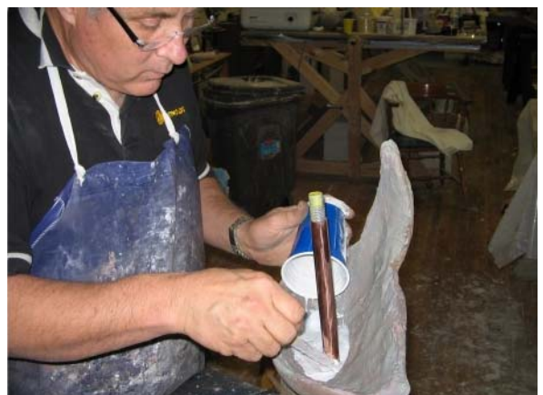
#14 Pouring in some plain Forton MG with fiberglass to secure the head to the connecting all thread and copper pipe.
