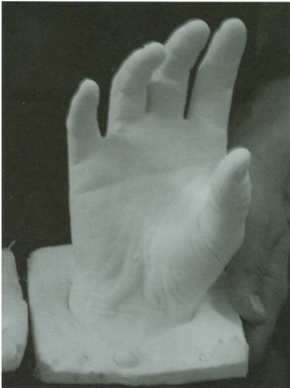
Lanryn's hand cast in urethane with Watertrap showing excellent detail.
