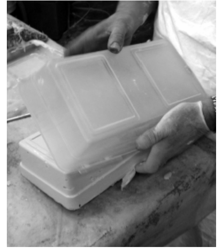
Waiting several minutes after the alginate gelled, the mold could then be removed.
