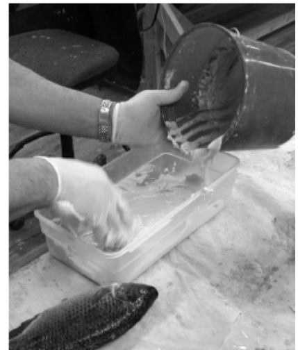
Pour the mixed alginate into the mother mold and smooth it out with your fingers.
