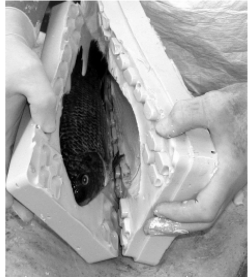
Once free of the mother mold, gently pull the top from the bottom to separate the mold halves.
