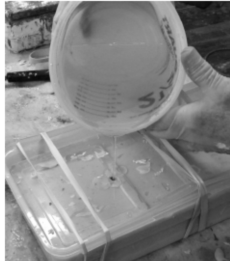
Fill the fish mold through the pour hole in the hole
