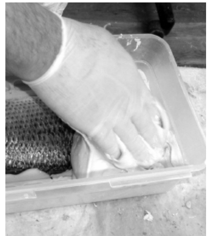
With the bottom layer gelled, mix and pour a top layer, nearly filling the mother mold.
