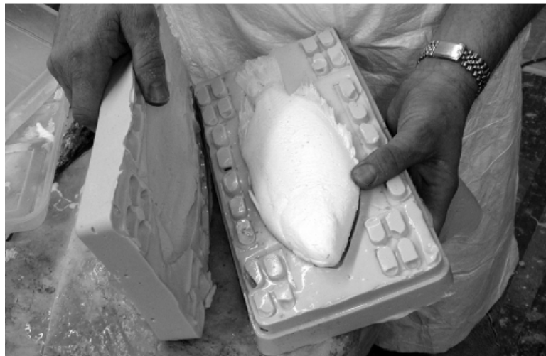
Once extra time has allowed thin areas to set up properly, separate the mold halves and remove your plastic fish.
