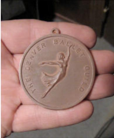
Photo #11. The medallion redone using the new technology. Notice the letters and the boarder. Shown here cast in resin with copper powder.
